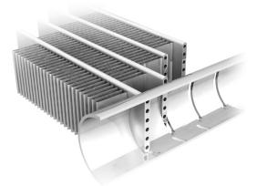
Already utilised in the automobile and aeronautical industries for many years, the MCHE micro-channel heat exchanger is entirely made of aluminium. This one-piece concept significantly increases its corrosion resistance by eliminating the galvanic currents that are created when two different metals (copper and aluminium) come into contact in traditional heat exchangers.
