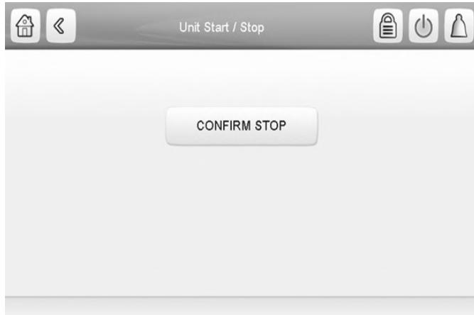
Confirm the unit shutdown by pressing **Confirm Stop** or return to the previous screen by pressing the
