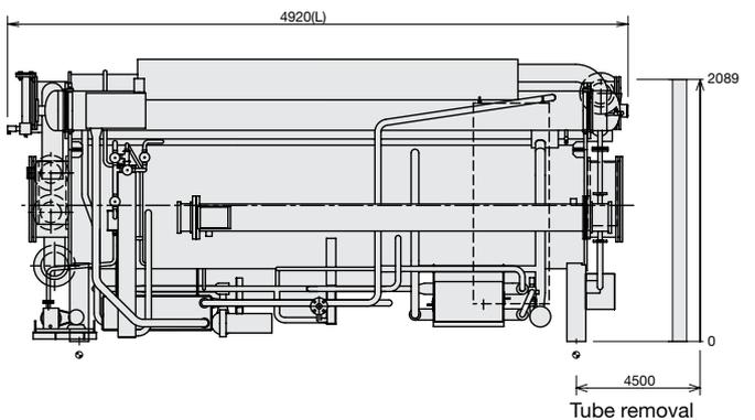
**NOTE: Dimensions are for guidance only. Refer to the certified drawings supplied upon request when designing an installation.**
