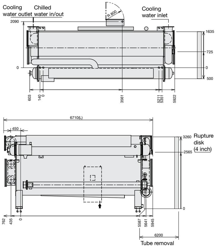
**NOTE: Dimensions are for guidance only. Refer to the certified drawings supplied upon request when designing an installation.**
