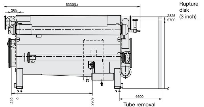
**NOTE: Dimensions are for guidance only. Refer to the certified drawings supplied upon request when designing an installation.**
