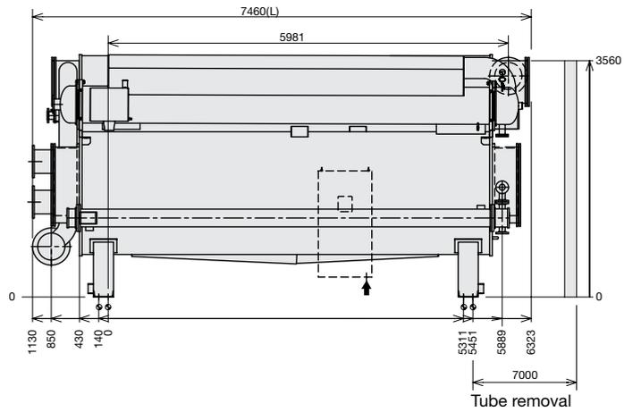
**NOTE: Dimensions are for guidance only. Refer to the certified drawings supplied upon request when designing an installation.**
