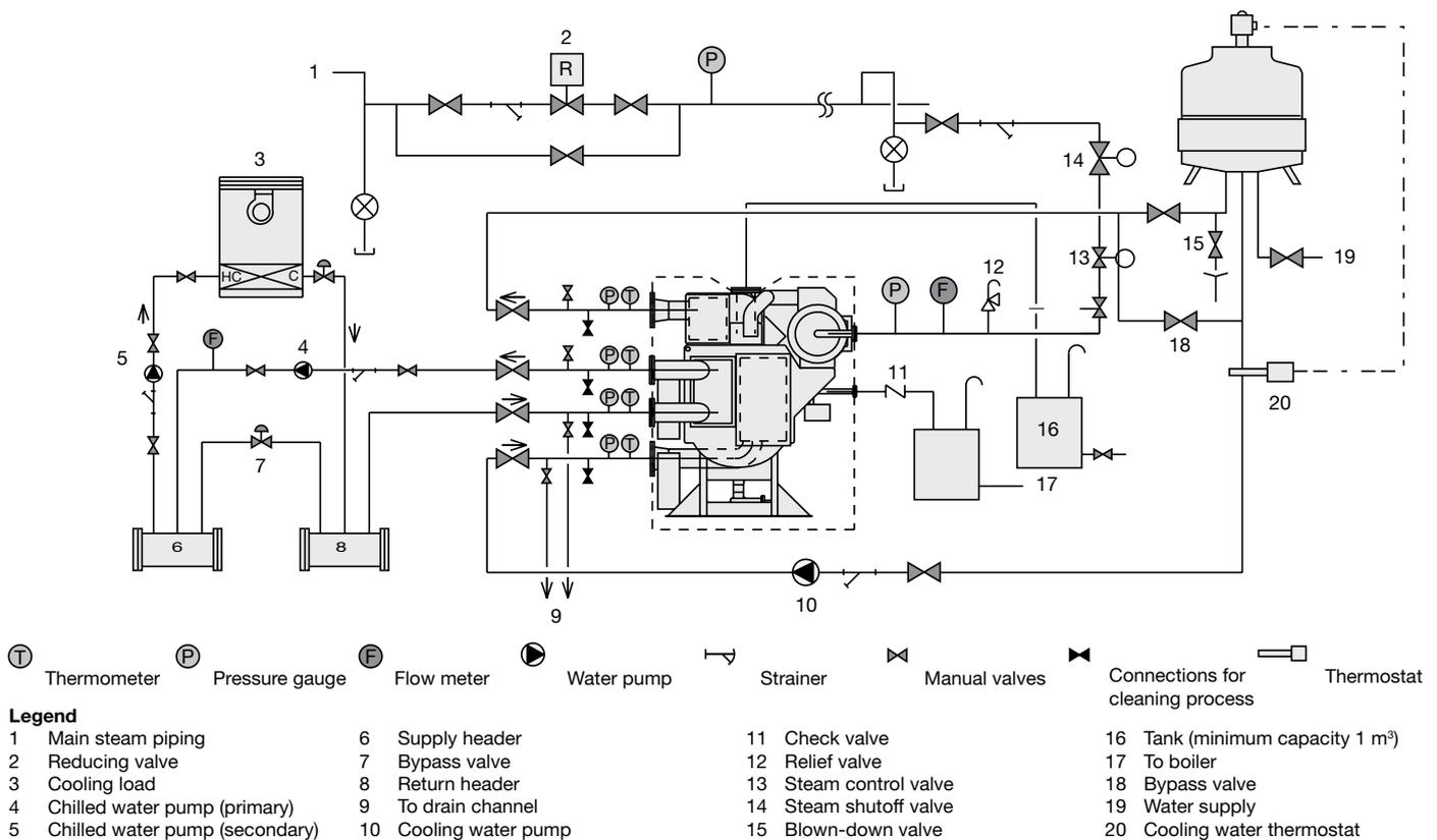
**NOTE:** In order to prevent freezing of the chilled water during the chiller dilution cycle, ensure continued operation of the chilled water pumps and cooling load until the dilution symbol on the control panel goes off. For the same reason the chilled water volume must be higher than 10.5 litres/kW.
