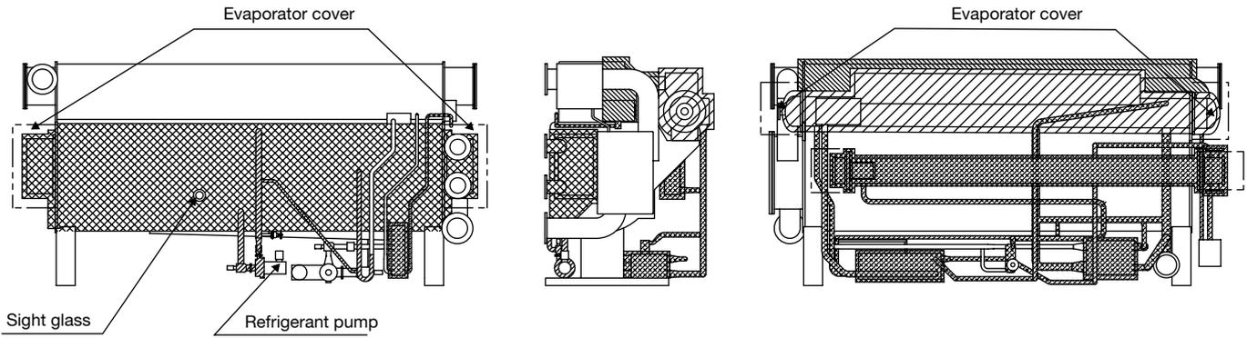
Fig. 32 - Insulation area 16NK-71 to 16NK-81
