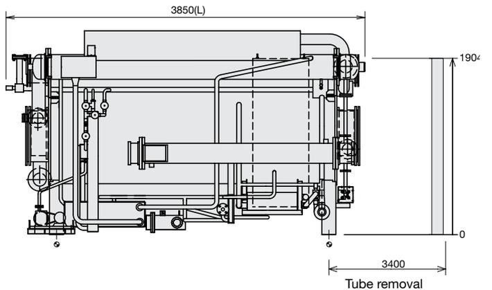
**NOTE:** Dimensions are for guidance only. Refer to the certified drawings supplied upon request when designing an installation.
