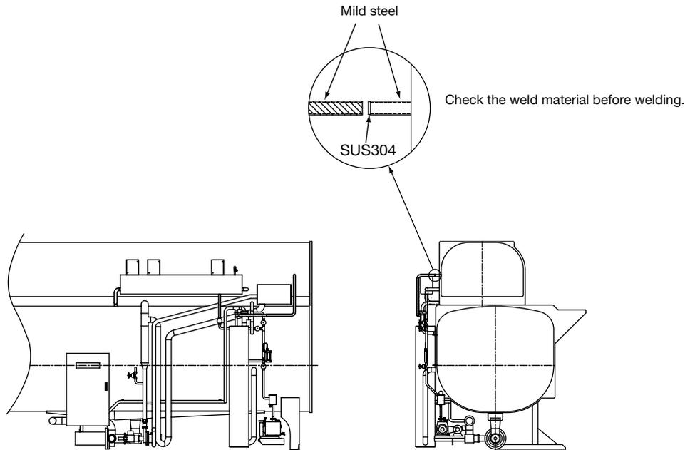
**4.4.3 - Assembly of the lower shell and the high-temperature generator**
