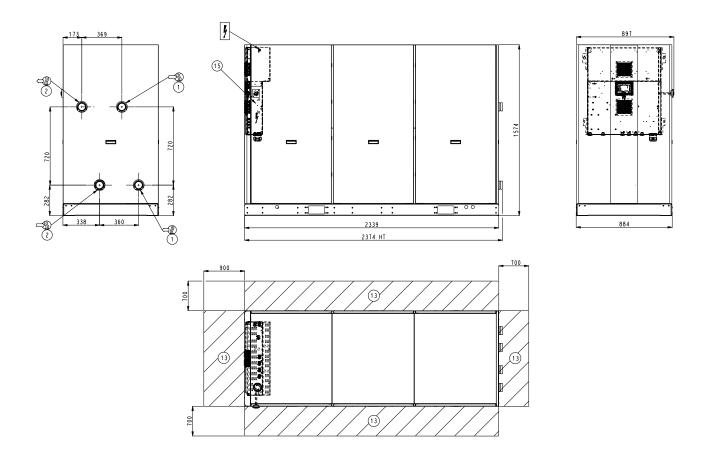
30WG 110-140 - unit with hydronic kit and top connections (option 116-270 and 274)
