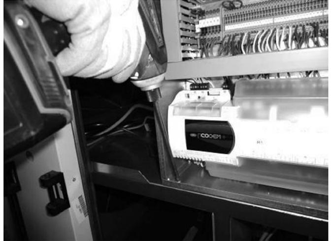
3. Move the electrics box; a sufficient length of cable is provided
